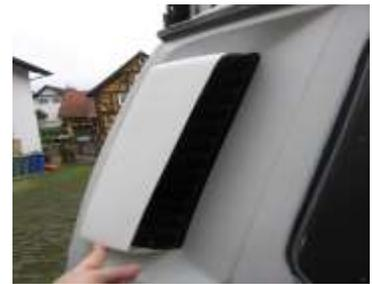
Put the original screw in the rear hole, put the air vent/scoop back in place, tighten the rear screw with the small ratchet. Insert and tighten the original front screw with the screw driver. Enjoy!
