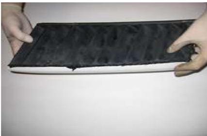
**Place the scoop over the vent and position the edges of the scoop in line with the edges of the vent. Try not to get the adhesive on the outside of the scoop.**
