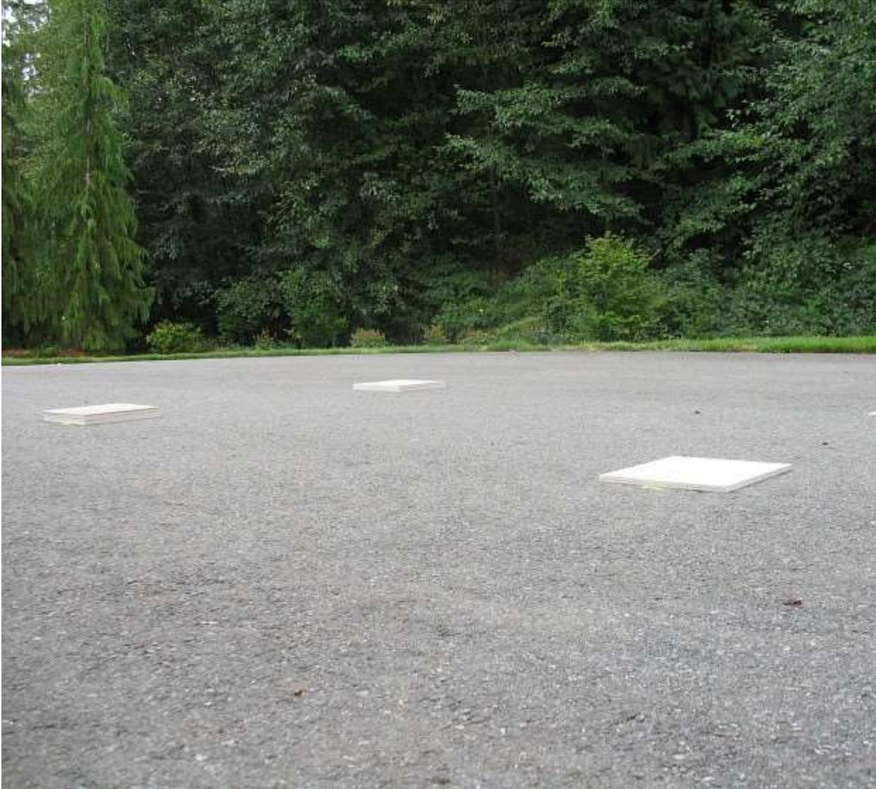
**Remember that I mentioned placing at least two shims in each tire location? This allows the last tile to swivel on the one underneath it as well as lets the suspension settle easier should you need to jack up the vehicle for access to the suspension components while adjusting things. Being able to rotate the wheels during the caster adjustment procedure is where this comes into play the most.**
