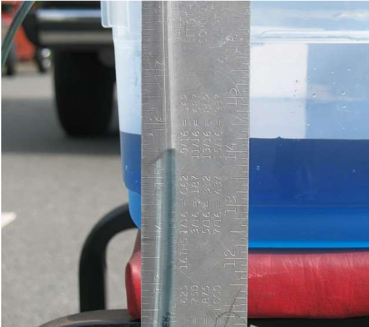
With the water level created, you can now place the end of the square in the middle of each of your shims to determine which location is the highest. Remember that the highest location will read the lowest number on the square. My highest location (left front) measured right at 15" on the square and my lowest location (right rear) measured 16 1/4".
