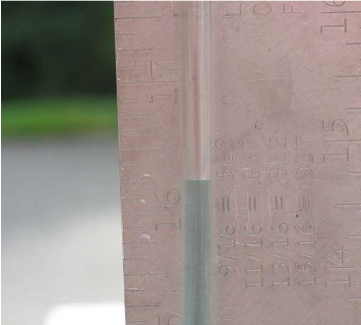
**Using the 1/8" thick tiles, I stacked them in the three lowest locations until I achieved a level of 15" on the square of my water level at all four locations. Since the tiles are 1/8" each, it was very easy to figure out how many were needed for each location.**
