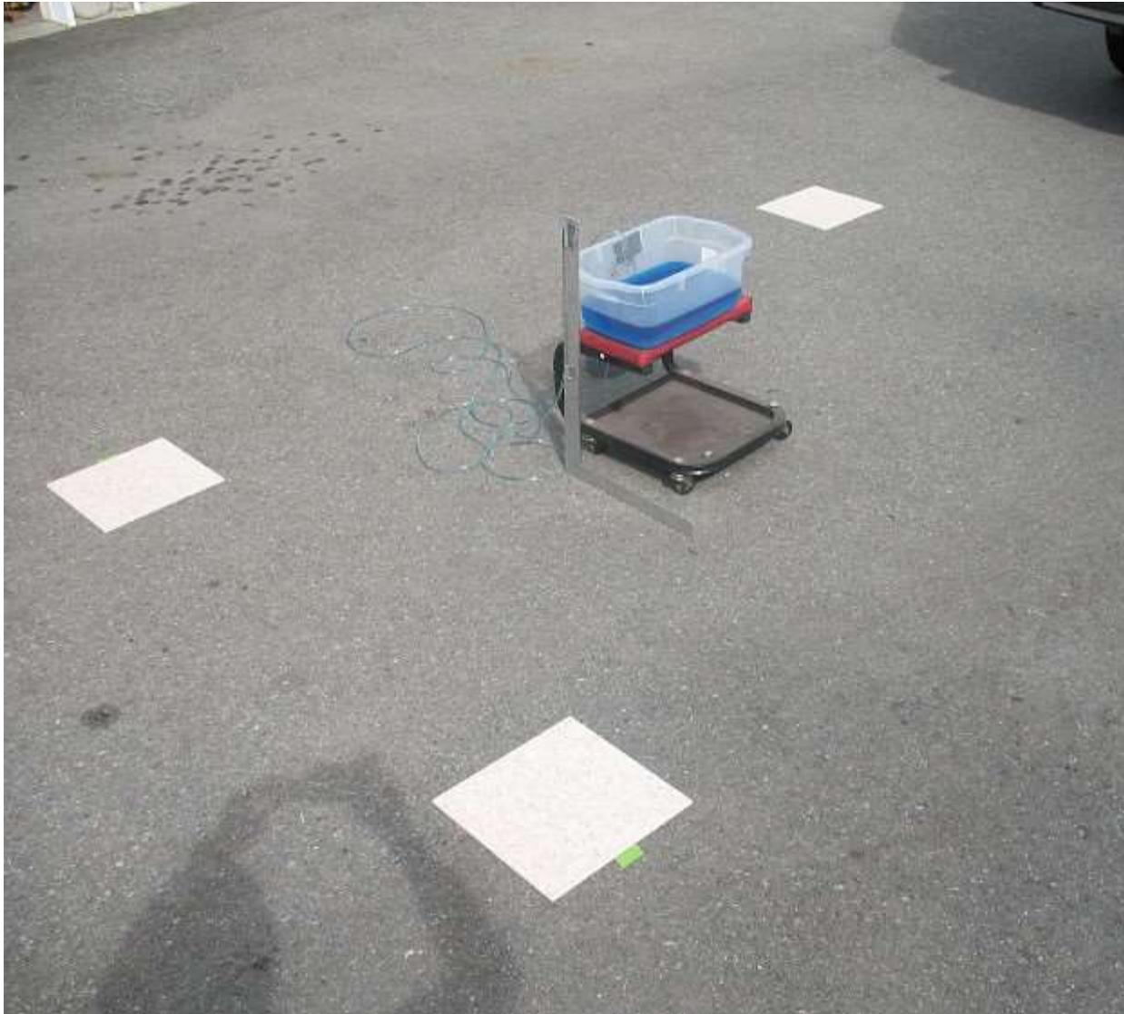
**Tape one end of the clear tubing into the water and secure it (duct tape) so that the end of the tubing remains submerged.**
