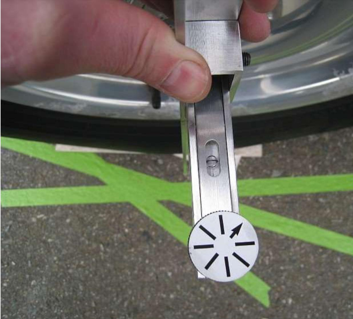
**With the number of marks accurately counted, you need to convert the number of marks to number of full turns of the knob. The knob has eight marks on it, so we just need to divide the total number of marks that we counted by eight. In my case,  $40 \div 8 = 5$ . In order to find out the angle of caster in degrees, we then have to multiply that last number by 1.5. So in my case, the complete number sequence looks like this:**
