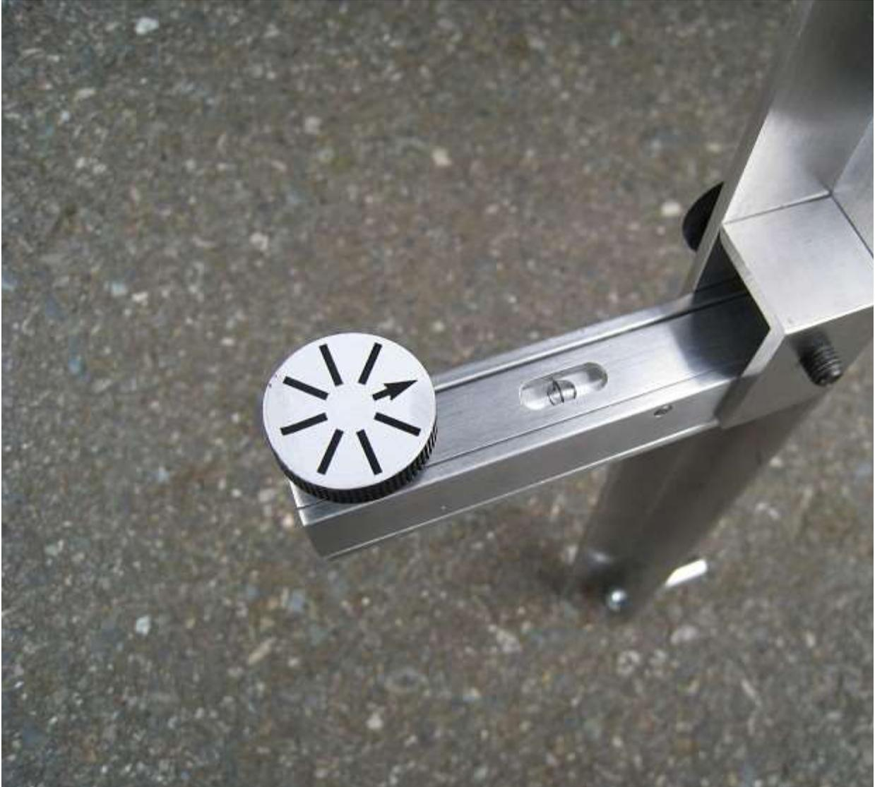
Then it is a simple matter of positioning the pegs on the tool onto the rim lips so that the tool is held vertically. Then turn the knob in the direction necessary to allow the bubble to be centered, counting the marks that it takes to do so. If you have to turn the knob counter clockwise to level the bubble, you have negative camber and if you have to turn the knob clockwise, you have positive camber.
