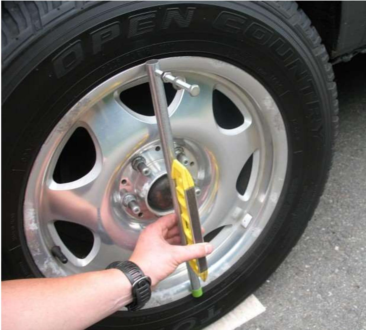
**Using the bar with the bubble level held tightly against it (taping the level to the bar helps), rest the bar up against the rim lips making sure that the bar points straight up and down. Adjust the bolt in the bar out until the bubble in the level shows perfectly level.**
