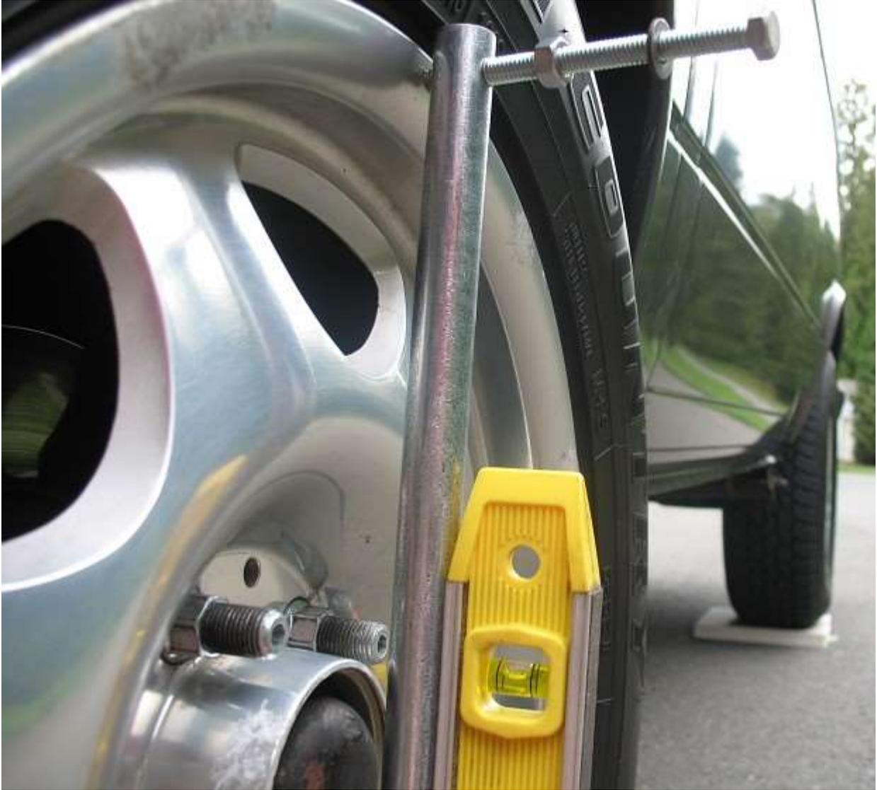
**Now it's just a matter of measuring how far that bolt sticks out past the edge of the bar and doing some calculations to find the camber angle.**
