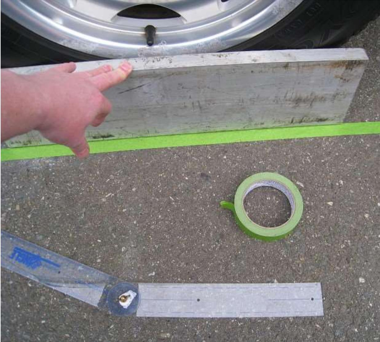
**Then you will need some type of tool that will help you indicate 20° to the first line on the ground. I used a 12" plastic angle finder. Turn the front wheel until the wheel is 20° to the first line as indicated by both the angle finder and the straight edge. Make a second line on the ground just like you did for the first. Now turn the wheel the opposite direction and repeat, making another line at 20° to the first line.**
