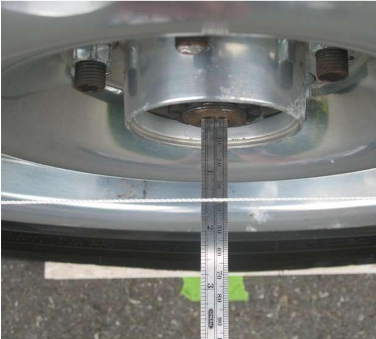
**Now we can move on to actually measuring the toe angle. Again, this is where the thrust angle can come into play. Toe angle adjustments can be performed without the use of the string jig. All it takes is a simple flat bar across each front wheel and a tape measure. Measure in front of the tire and in back of the tire. The difference is your toe angle. There are two problems with this method.**
