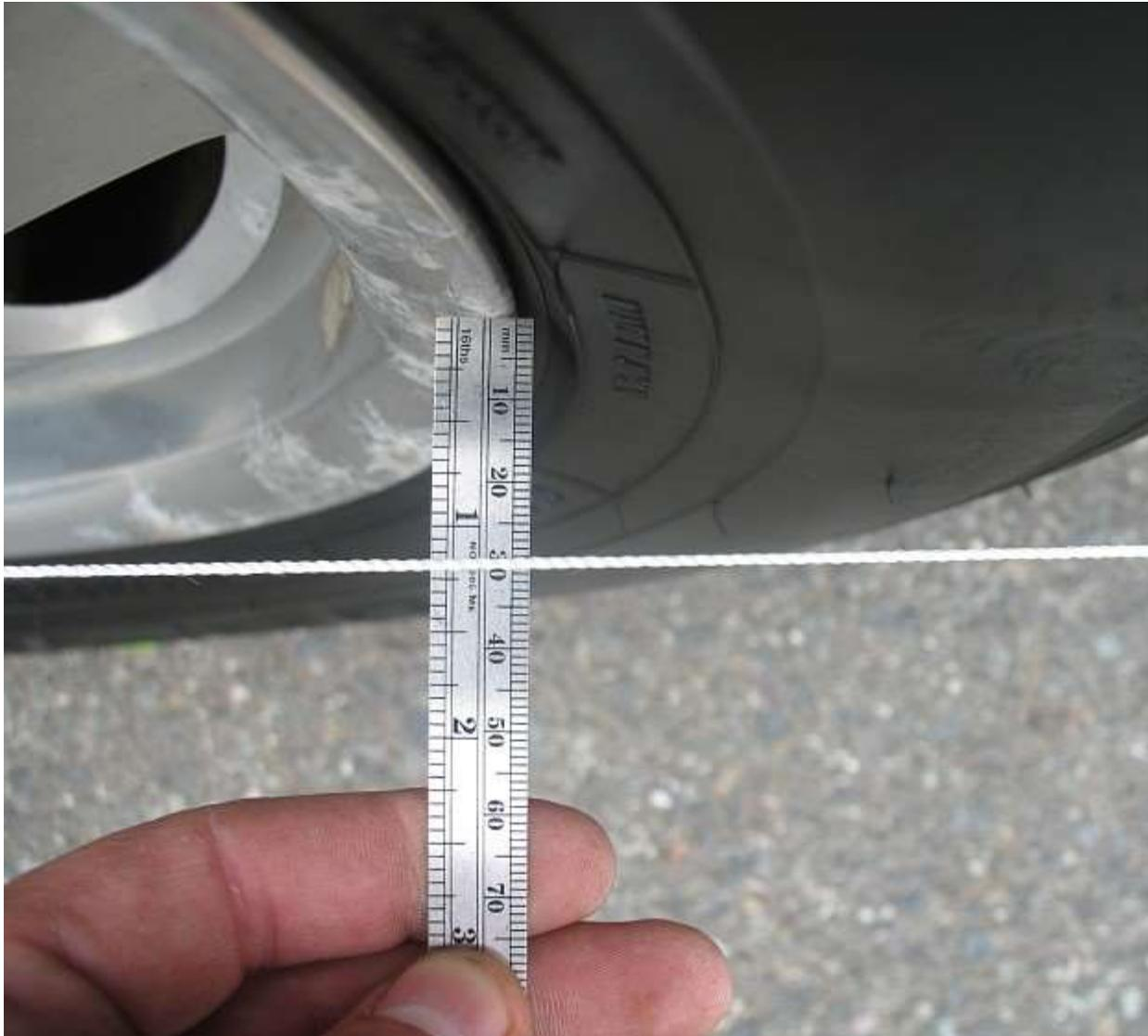
The pictures below show the real world measurements of the right rear wheel of my van. You can see that both front and rear lips measure 37mm (actually one of the photos looks like 37.5mm, but the ruler is angled slightly making it look that way. Taking pictures while holding rulers is hard) resulting in zero toe angle for the right rear.
