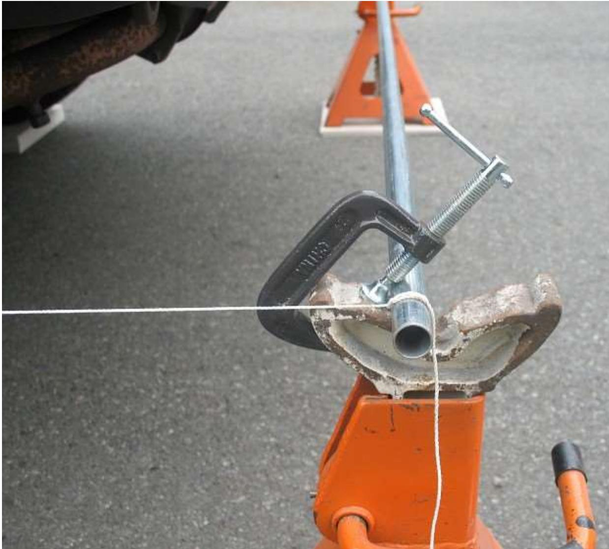
**With the strings in place, you will now need to raise or lower the position of the conduit in order to position the string at the exact centerline of the wheel hubs. Again, use whatever means you have to accomplish this. Refer to the photos above for two different approaches.**
